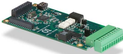
Current Loop Card Current Loop/RS485/RS422.
